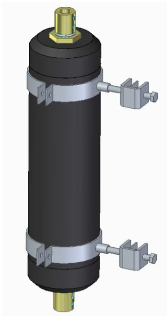
Figure 10. Clamps and attachment to dinfil filter legs.
