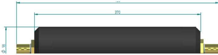
Figure 3. Measurements of the dinfil ground filter DNNFT model.
